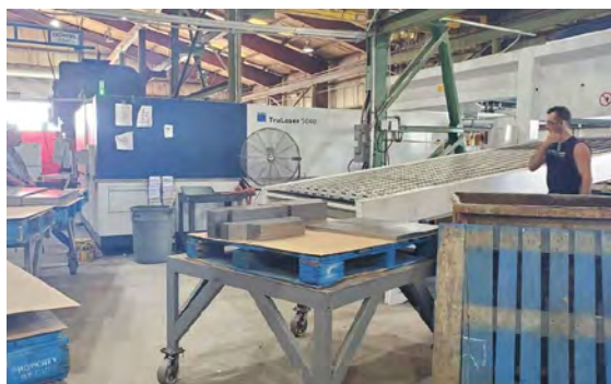
Miller Metal Fabrication’s TRUMPF 10-kW TruLaser 5040 has added new laser cutting capacity for the fab shop. Images provided by Miller Metal Fabrication
